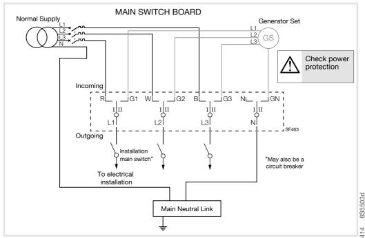
This modular changeover switch is not a disconnector. The isolation must be ensured with an appropriate device. The changeover incoming must be protected against short circuit with an appropriate MCB 63A - 6kA - C curve.
