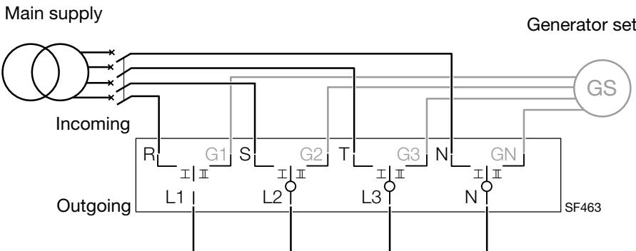
**(EN)** This modular changeover switch is not a disconnector. The isolation must be ensured with an appropriate device. The changeover incoming must be protected against short circuit with an appropriate MCB 63A - 4,5kA - Curve C.
