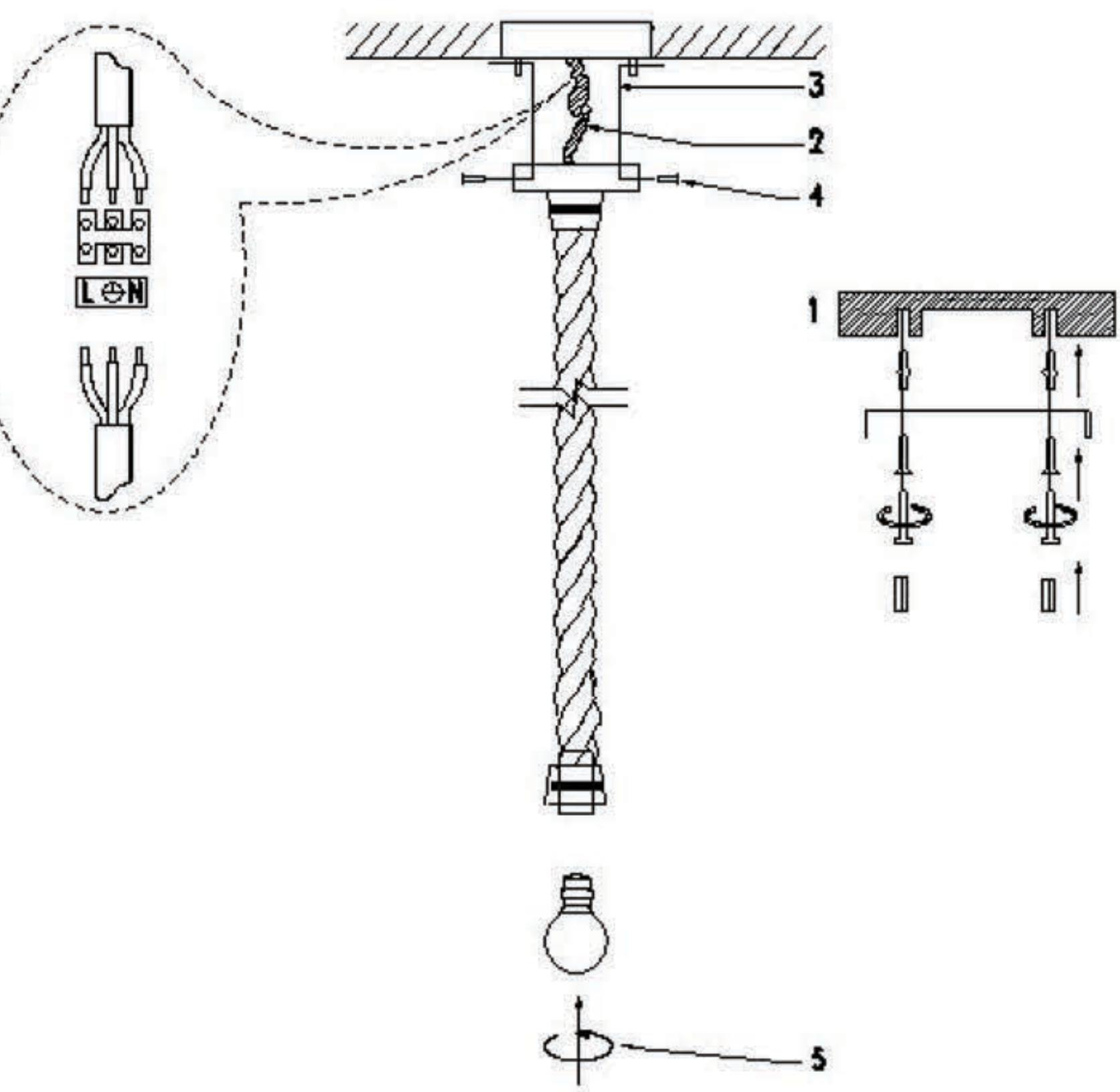
1. Use screws to fix mounting bar to the junction box.
