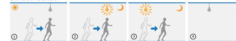
1. When the ambient light is bright enough, even if a moving object is detected, the lamp will not automatically light up
