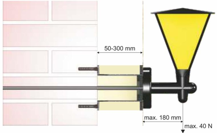
There is necessary to cut the carrier including inserted insulation before installation depending on layer thickness insulation.
