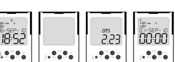
Performed by shortly pressing the hidden RESET button with a blunt-pointed object (e.g. a pencil or screw-driver with a diameter of at most 2 mm).
