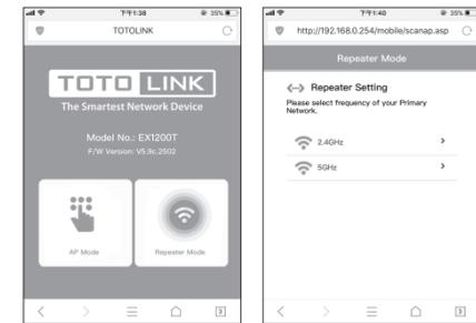
2. Select your router's 2.4GHz and 5GHz primary network and enter the password, then click "connect". It indicates successful connection when the 2.4G/5G green LED remains solid on.
