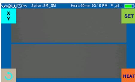
③ Selected heat mode appears on the screen. Press [R] button to return to initial interface.
