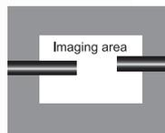
Fiber ends visible on the monitor.
