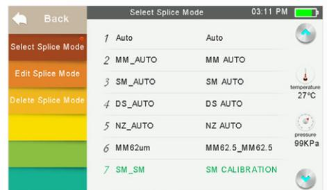
③ Selected splice mode appears on the screen. Press [Reset] button to return to initial interface page.
