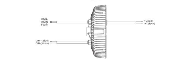
• Contact DIM+and DIM- with 1-10V dimmer
